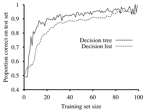
Figure 18.12 Learning curve for DECISION-LIST-LEARNING algorithm on the restaurant data. The curve for DECISION-TREE-LEARNING is shown for comparison.
